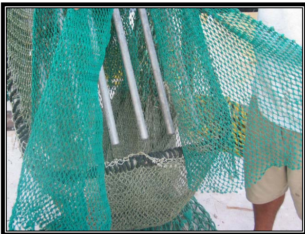
Fisheries Officer inspecting the TED on a shrimp trawler
